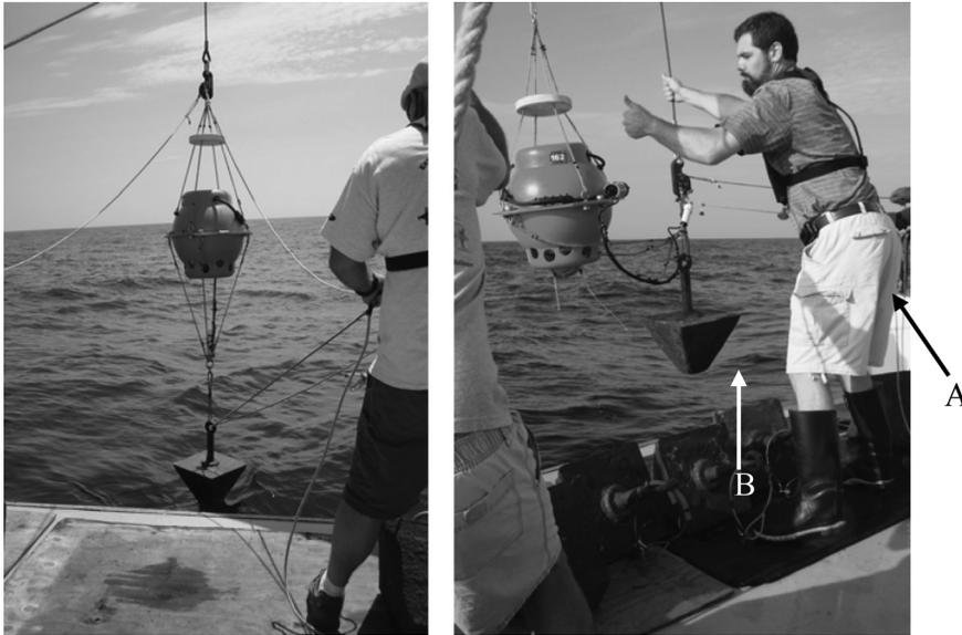
FIG. 4. Deployment of pop-ups during the GMI NJDEP project. The left photograph depicts a pop-up being deployed with the acoustic burn release by-passed. The right photograph presents a unit being deployed with the burn unit engaged (A) and a GPS tracking system (B) attached to the pop-up.
