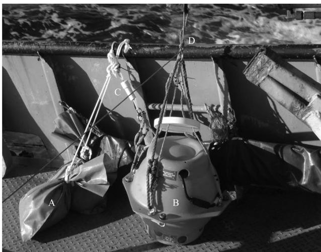
FIG. 2. Pop-up rigged prior to deployment in Icelandic water. A denotes the weight (sand/gravel bag). B is the pop-up. C is the acoustic release unit. D is the rigging used to deploy the pop-up.
