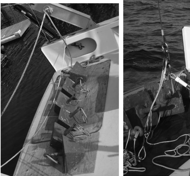
FIG. 11. Steel cabling replaced the nylon looped webbing for the GMI NJDEP pop-up deployments. The left image shows five anchors each with steel cable attached. The right image shows the burn unit of one pop-up attached to the steel cable then the anchor.
