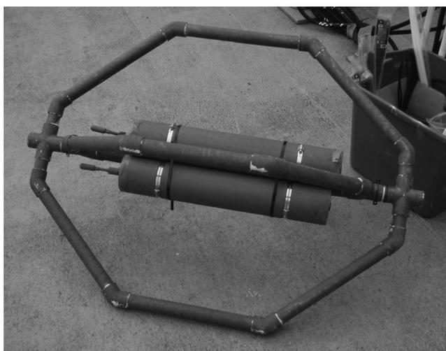
FIG. 9. PVC housings with DSG recorders and battery packs, attached to the center post of a protective PVC cage (pre-deployment). Note that the recorder housings are held to a protective cage with both stainless hose clamps and large tie wraps.
