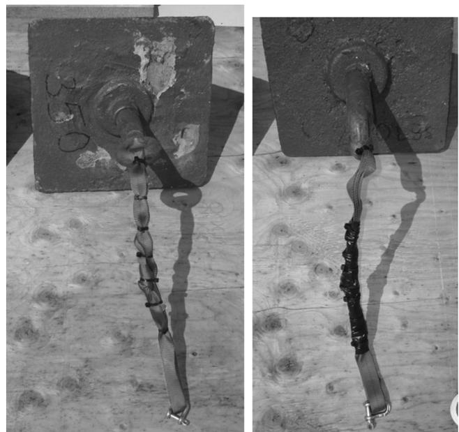
FIG. 3. Anchor rigging used during five deployments during the GMI NJDEP project. The left image shows the webbing prior to tape application; the right image depicts the rigging ready to deploy.
