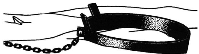
FIG. 6. P-ring used for anchoring for T-POD and C-POD units. The two spikes on the underside of the iron ring prevent the ring from being dragged sideways. Even on hard sand bottoms this anchoring can withstand very high pulls in the horizontal direction. To prevent entanglement, the first 2 m of chain can be covered in plastic tubing.
