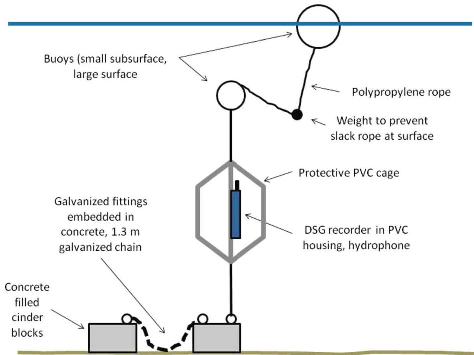
FIG. 10. (Color online) Modified mooring design for the 2009 for the DSG recorder deployments.
