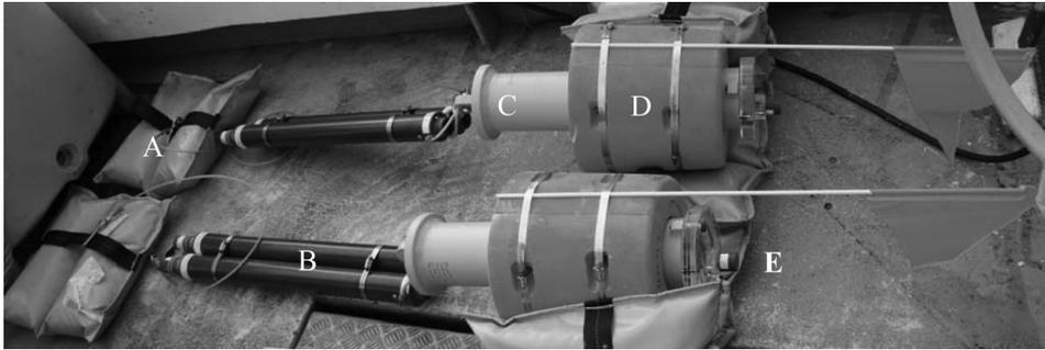
FIG. 1. EARs prepared for deployment. (A) Weight for mooring of the unit, 3–4 sandbags are used for each unit. (B) Two acoustic release units. (C) EAR unit. (D) Syntactic foam float collar (color is often bright orange). (E) Hydrophone.
