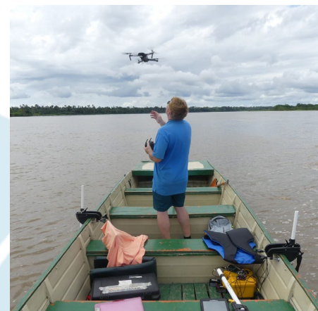
T. Dillen deploys a drone while a low frequency array records audio off port (left) and a high frequency array records off starboard (right).
